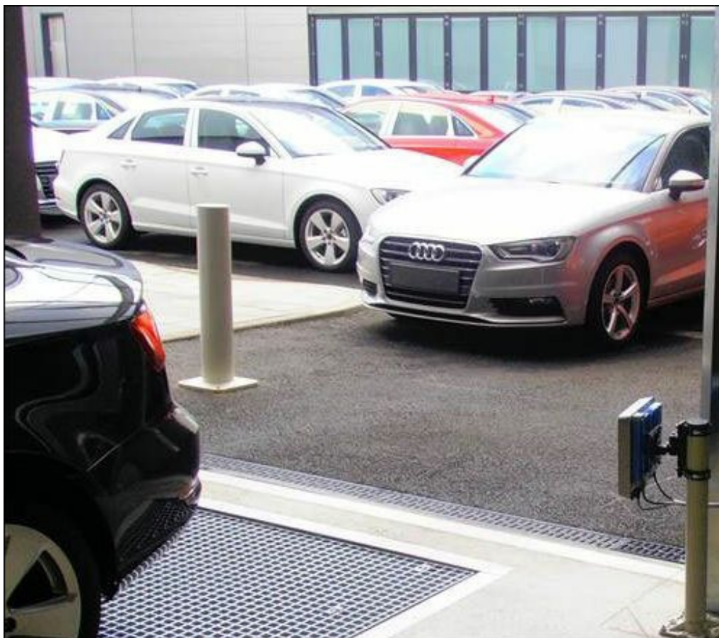
An RFID reader records each vehicle's entry to the technical inspection area.
