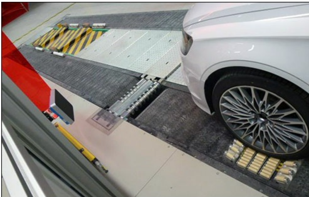
At each station in the finishing area, an RFID reader captures the ID number of the vehicle's tag, thereby documenting which processes have been carried out.
